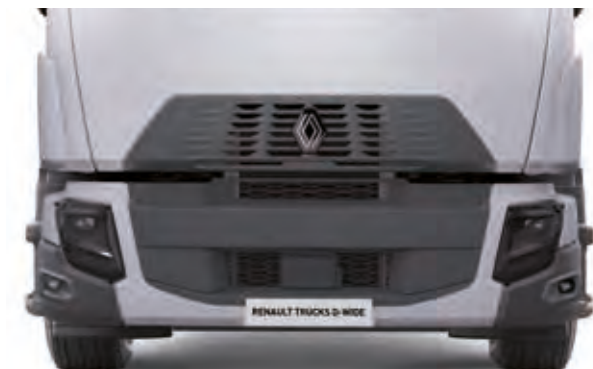
PLASTIC BUMPER (D WIDE) WITH STEEL CORNER PIECES available as standard.
