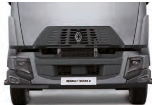
PLASTIC BUMPER (D) WITH STEEL CORNER PIECES available as standard.
