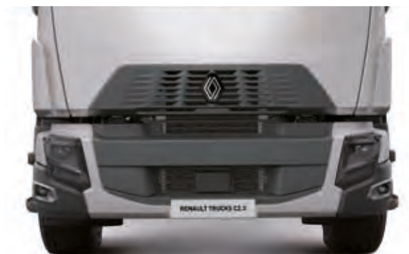
PLASTIC BUMPER (C 2.3) WITH STEEL CORNER PIECES for greater resilience.
